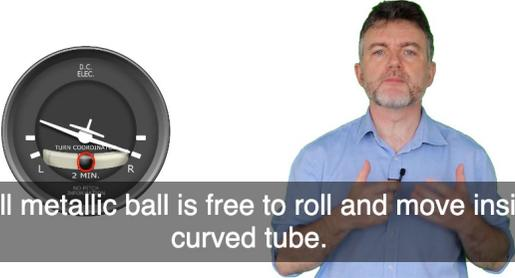
a small metallic ball is free to roll and move inside a curved tube.
